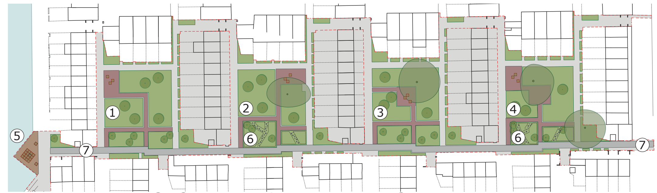
Proposed landscape layout ① - ④ Courtyards, ⑤ - Lakeside Feature, ⑥ - Swales, ⑦ - Portmeadow Walk
